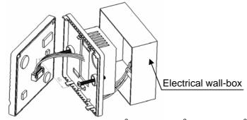
Screw terminals for 2 x 1.5 mm $^2$  or 1 x 2.5 mm $^2$ , min. ( 0.5 mm $^2$  )
